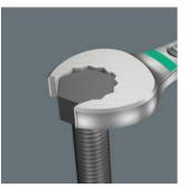
The double hexagon geometry on the mouth and ring sides secures the positive connection with the screw head or bolt and reduces the risk of slipping.
